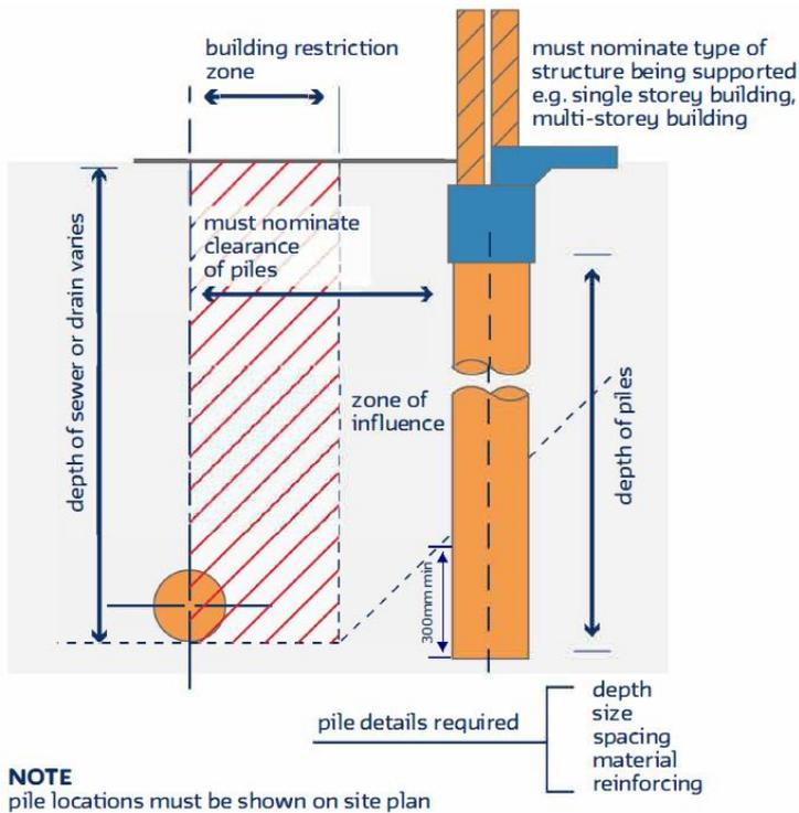
**Figure 5 Example pile detail**
