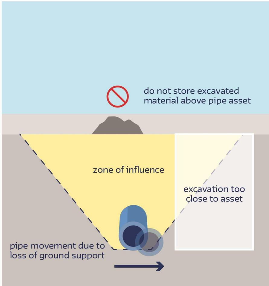
**Figure 14 Open excavations – not acceptable**
