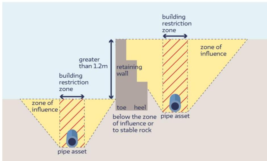
**Figure 10 Retaining walls**
