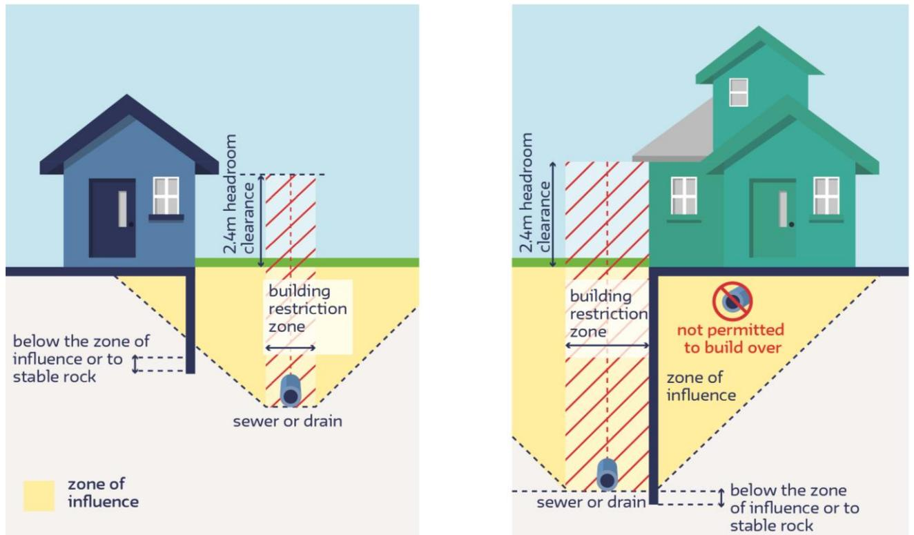
**Figure 2 Single storey buildings (left) and multi-storey buildings (right)**
