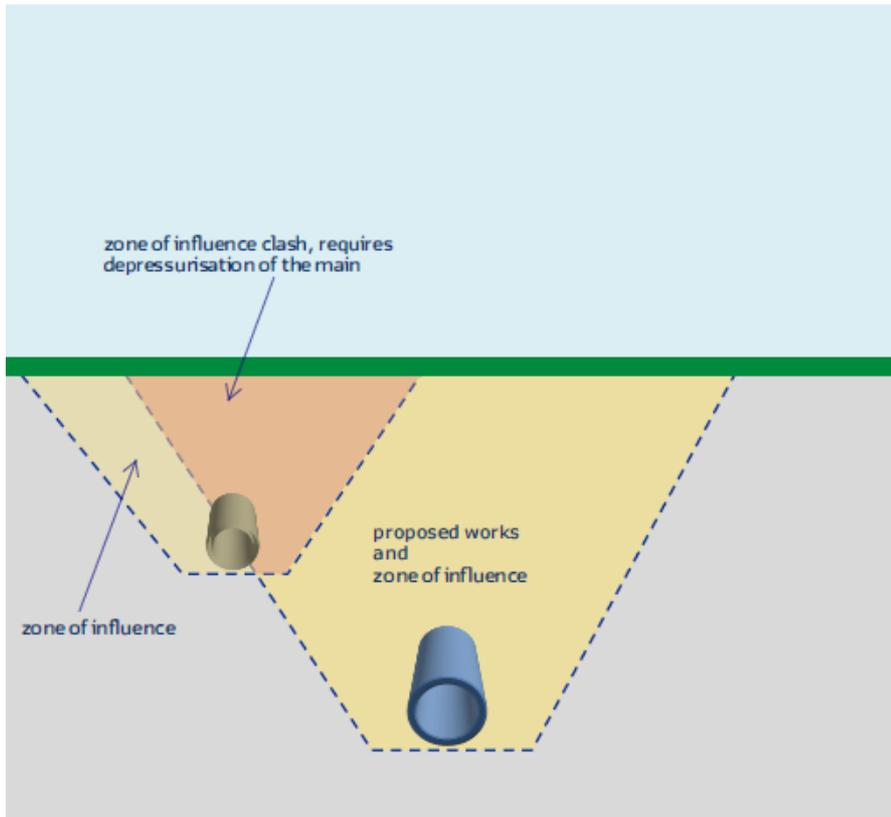
Figure 13 Open excavations – circumstances for depressurisation
