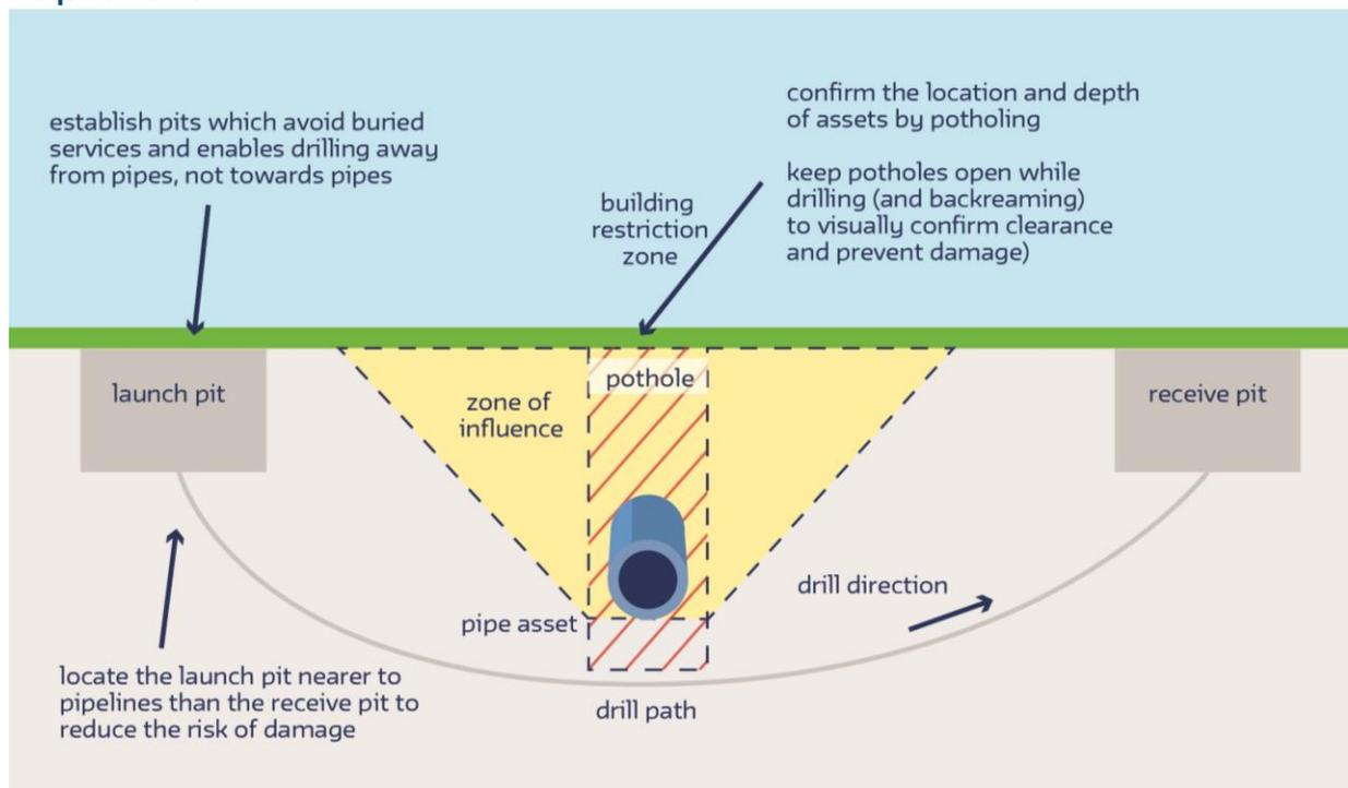
**Figure 16 Trenchless excavations**
