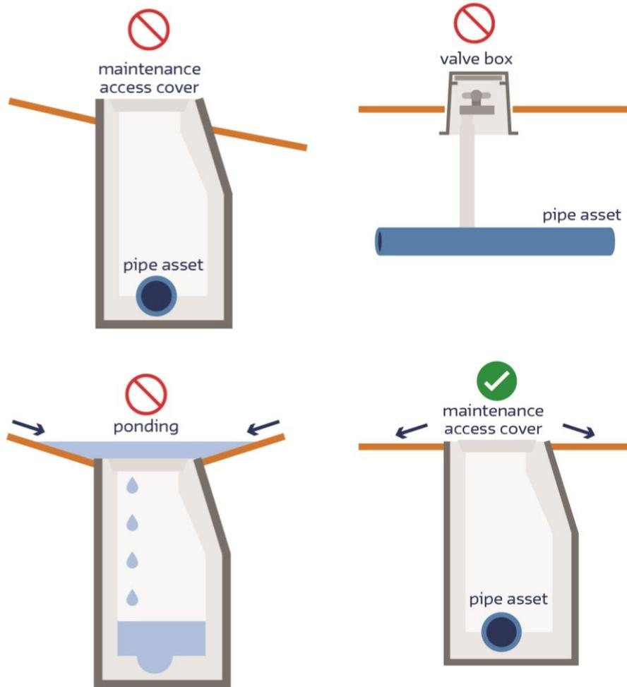
**Figure 2 Alteration of surfaces around covers and lids**
