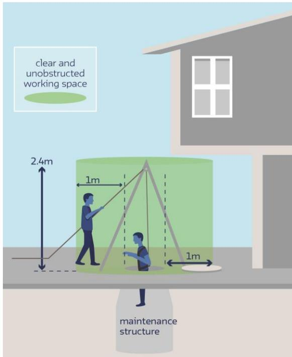
**Figure 3 Access clearances around sewer and drain maintenance structures**
