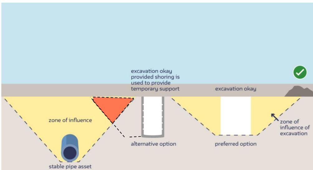
**Figure 15 Cont. Open excavations – acceptable**
