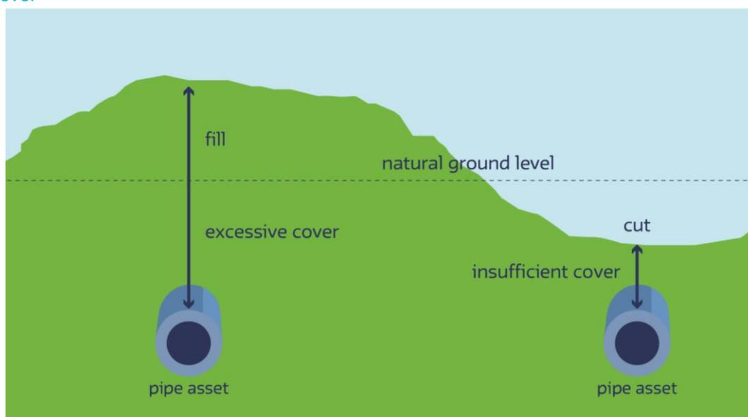
Figure 11 Earthworks and alteration of surfaces
